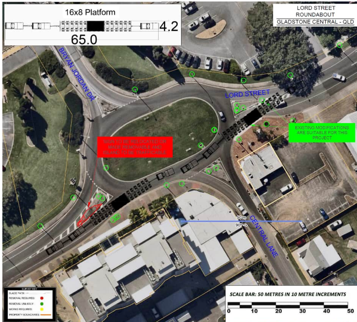
Figure 23 - Lord Street through roundabout at the intersection of Bryan Jordan Drive in Gladstone
