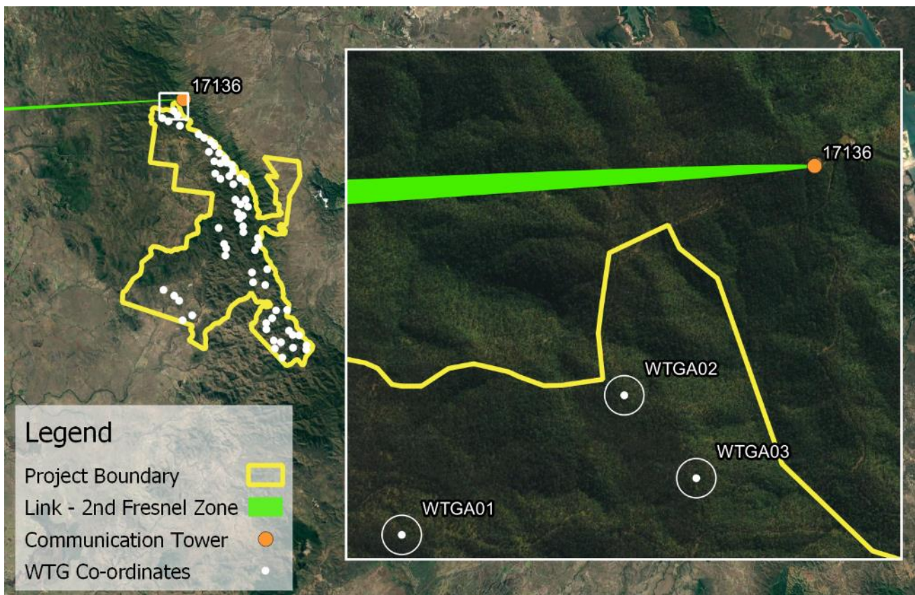
Figure 3.13 Point-to-point Link 10, calculated 2 nd Fresnel zone
