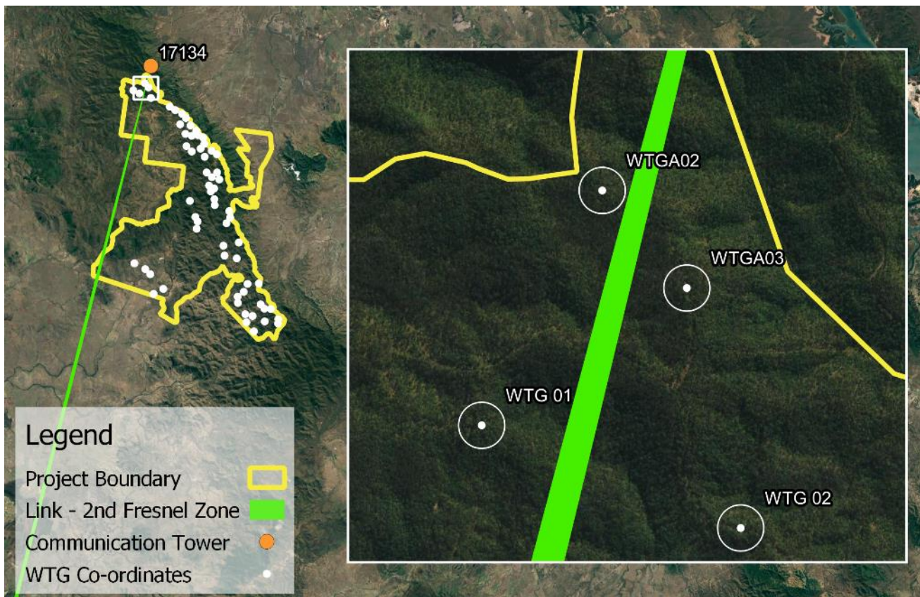
Figure 3.4 Point-to-point Link 1, calculated 2 nd Fresnel zone
